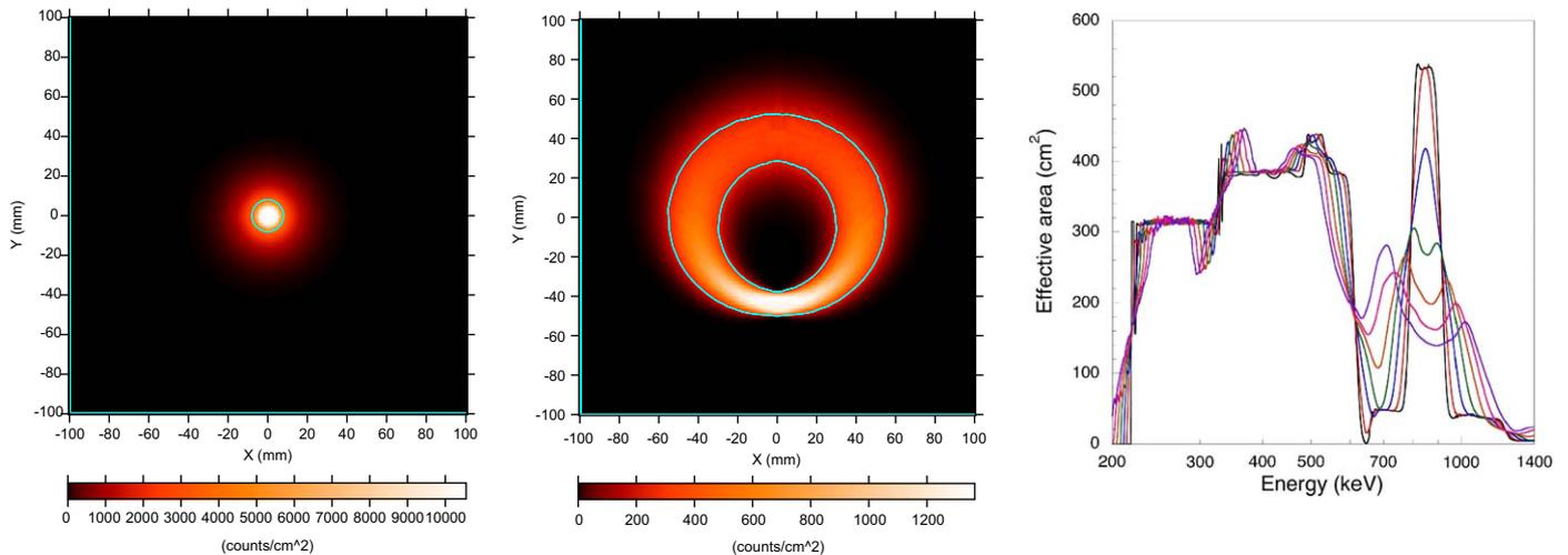
**Fig. 3.** Evolution of both spatial and spectral response of the high-energy band (~800–900 keV) of GRI Laue lens. Left and center panels show, respectively, the point spread function when the source is on-axis and 90 arc off-axis. Right panel shows the effective area of the lens for a point source moving in the field of view; from on-axis to 3 arc min off-axis by steps of 0.5 arc min are represented.
