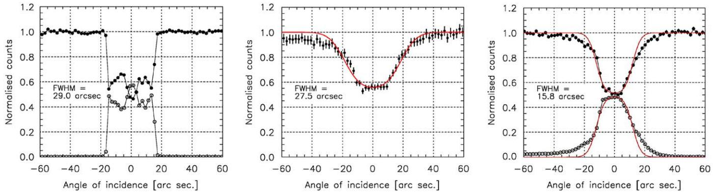
**Fig. 2.** Left: RC of a 23 mm thick SiGe gradient crystal measured at 300 keV (reflection 111). Center: RC of a 8.6 mm thick Cu crystal (220 reflection) realized at 489 keV. Right: RC of a 2 mm thick Au crystal (reflection 111) realized at 588 keV. Applying the transmission coefficient due to the absorption through the crystal, the achieved reflectivities are respectively: 0.26, 0.24 and 0.31. All these measurements have been performed at ESRF (Grenoble, France) on beamline ID15A.
